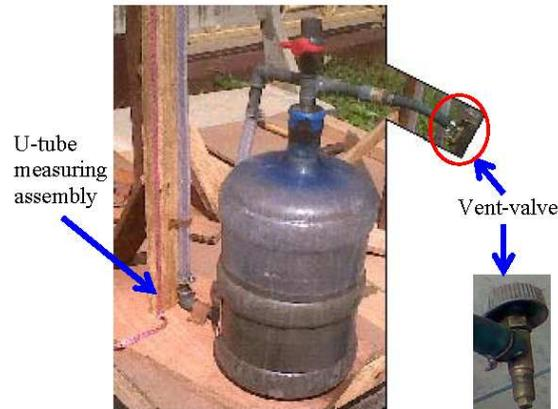
**Figure 1** Experimental set-up for bio-digester reactor with vent-valve and measuring U-tube assembly.
