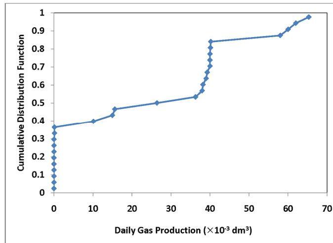
**Figure 3** Plot of the cumulative distribution function of the logistic fittings of daily gas production from substrate of *B. Primigenius*.
