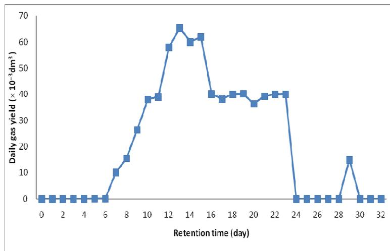
**Figure 2** Daily yield of gas production from the substrate of *B. primigenius* for 32 days retention time.
