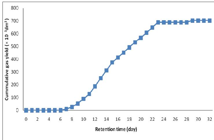
**Figure 4** Real-time cumulative gas production of *B. primigenius* substrate in fish-water medium.
