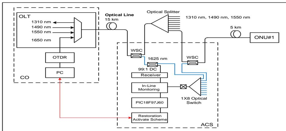
**Figure 2** Schematic diagram of the proposed surveillance and protection-based approach for link failures over FTTH-PON with an excellent combination of ACS and SANTAD.
