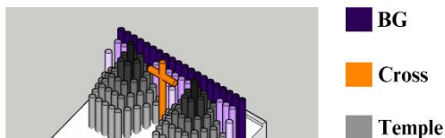
Figure 3. Basic Arrangement scheme of sonic crystals.
