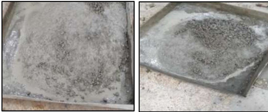
Figure 3 Segregation phenomenon at w/c = 0.57 and w/c = 0.615 .
