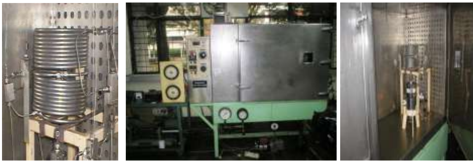
Figure 1 Slim tube apparatus (manufactured at Robinson Inc., Canada. Details are given in Table 2. The jacket was manufactured at ITB).
