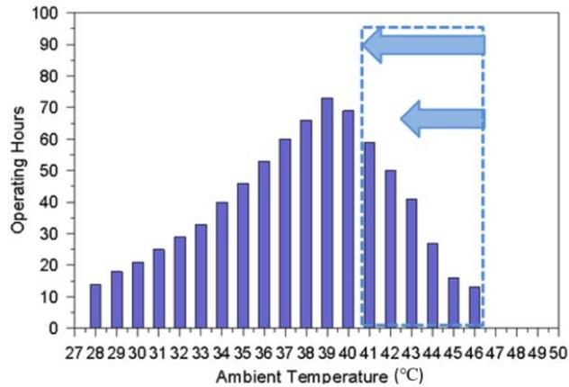
**Figure 7** Variation of the number of operating hours with ambient temperature in July.
