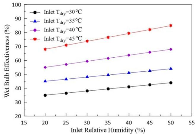
**Figure 11** Effect of inlet relative humidity on wet bulb effectiveness.
