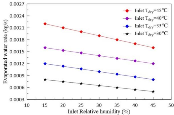
**Figure 9** Effect of relative humidity on water evaporation rate.
