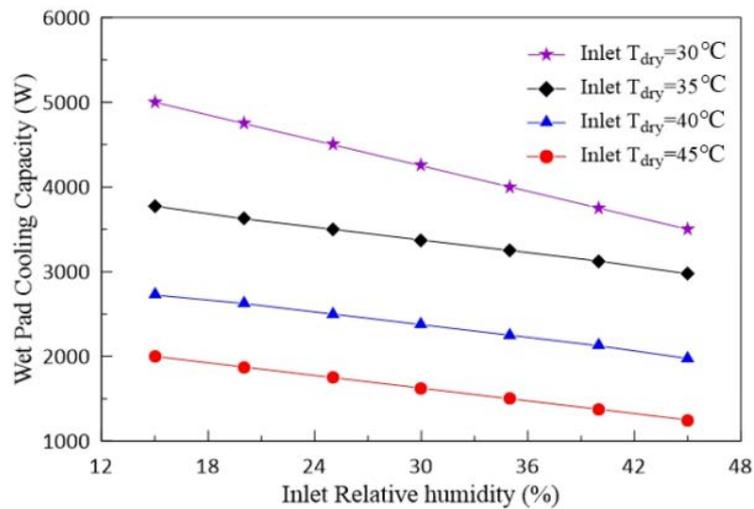
**Figure 10** Effect of relative humidity on the cooling capacity of the cooling pad.
