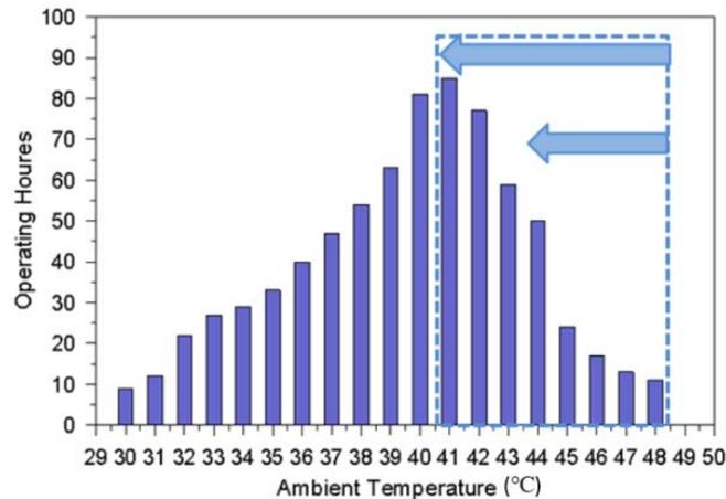
**Figure 8** Variation of the number of operating hours with ambient temperature in August.
