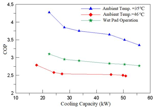
**Figure 12** Effect of relative cooling capacity on coefficient of performance (COP).
