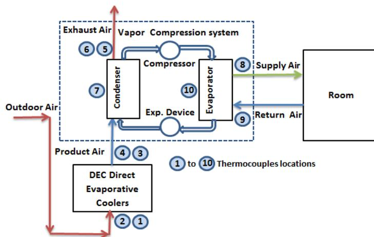
**Figure 1** Schematic drawing of vapor compression cooling system with direct evaporative cooler.
