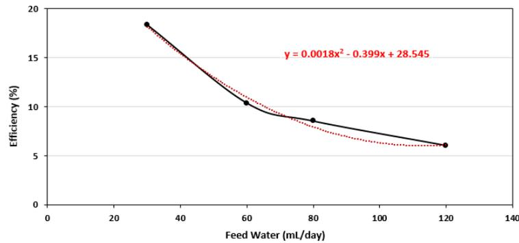
**Figure 6** Effect of using different feedwater quantities on still efficiency.
