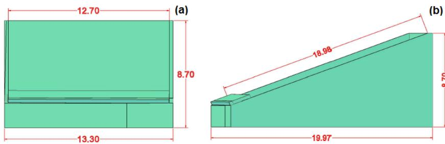
**Figure 2** The designed solar still: (a) front view, (b) side view.
