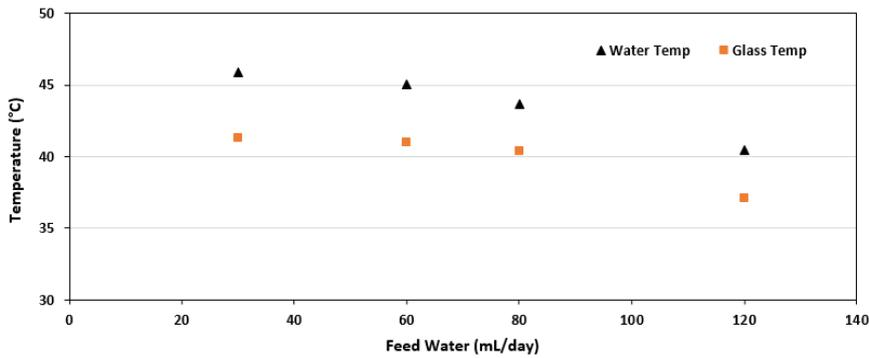
**Figure 5** Effect of using different feedwater quantities on the average temperature difference.
