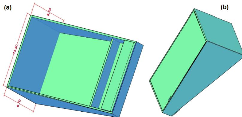
**Figure 3** Isometric 3D shapes of the designed solar still showing the principal elements (top, bottom, slope, front, back, and partition glass): (a) 3D reverse side dimensions, (b) 3D reverse side view.
