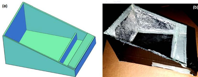
**Figure 4** The designed solar still: (a) AutoCAD 3D shape, (b) constructed 3D shape.
