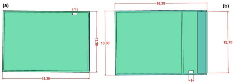
**Figure 1** The designed solar still: (a) bottom view, (b) top view.
