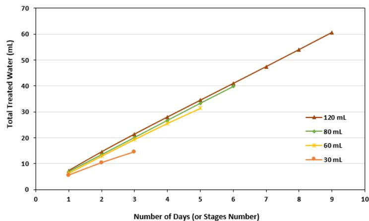
**Figure 7** Estimated number of days (or stages) required to treat 50% of different feedwater quantities in mL.
