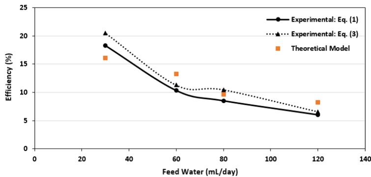
**Figure 8** Experimental and theoretical modeled efficiencies for different feed quantities.
