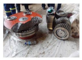
Figure 1 Smashed gearbox of a jack-up device.
