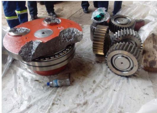
**Figure 1** Smashed gearbox of a jack-up device.
