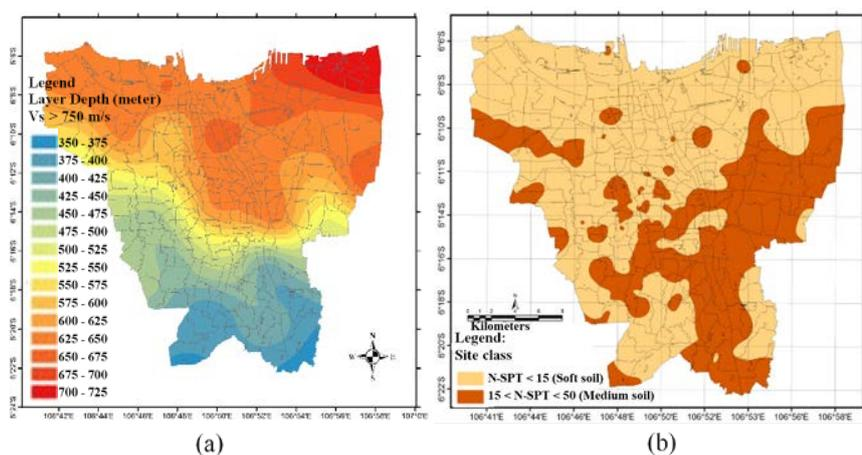
**Figure 1** Contour map of Jakarta: (a) depth of bedrock based on microtremor array measurement conducted by Ridwan *et al.* [4], (b) site classification based on SNI-1726-2012 by Irsyam *et al.* [3].
