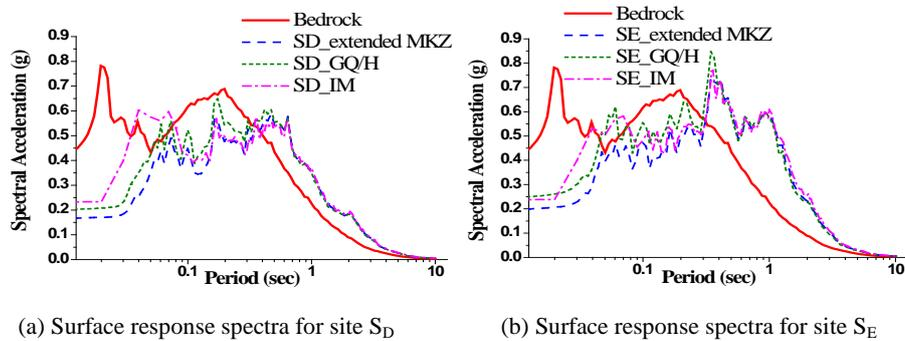
**Figure 6** Surface response spectra of the three soil models for a megathrust earthquake with a return period of 2500 years scaled at spectral period of 0.0 s.
