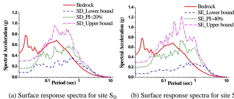
**Figure 11** The effect of boundary curves of  $G/G_{max}$  and  $D$  on the surface response spectra due to a megathrust earthquake with a return period of 2500 years scaled at a spectral period of 0.0 s.
