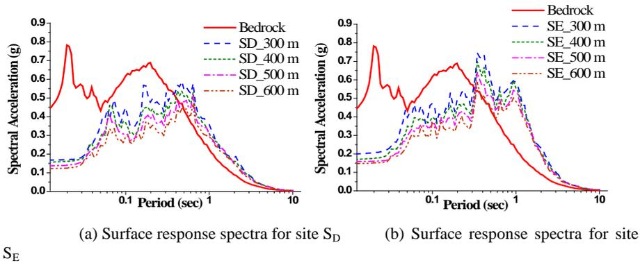
**Figure 7** The effect of depth of bedrock on the surface response spectra for a megathrust earthquake with a return period of 2500 years scaled at a spectral period of 0.0 s.
