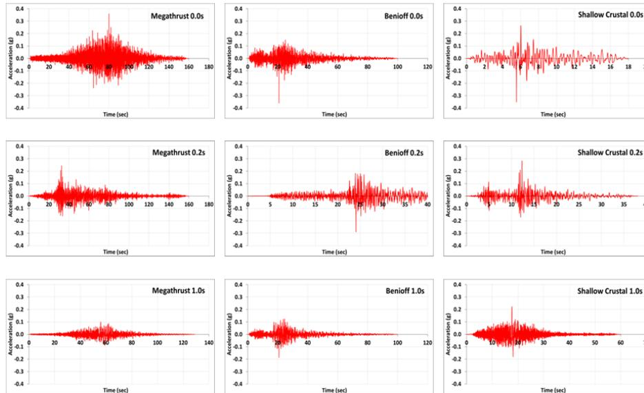
**Figure 4** Modified acceleration time histories on bedrock for Jakarta from megathrust, benioff, and shallow crustal earthquake sources for a return period of 2500 years (modified from Delfebriadi, *et al.* [22]).
