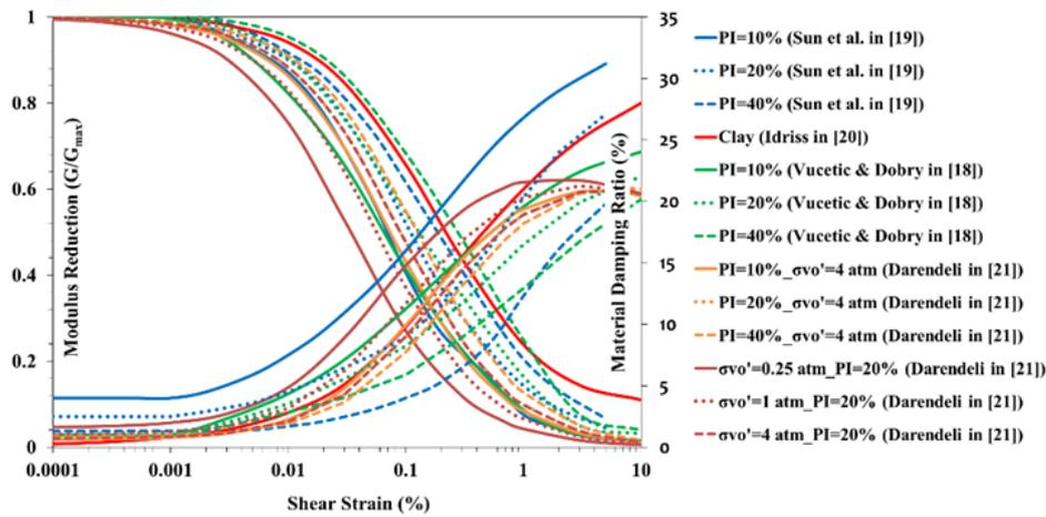
**Figure 3** Curve models of shear modulus reduction and damping ratio for cohesive soils from several references.
