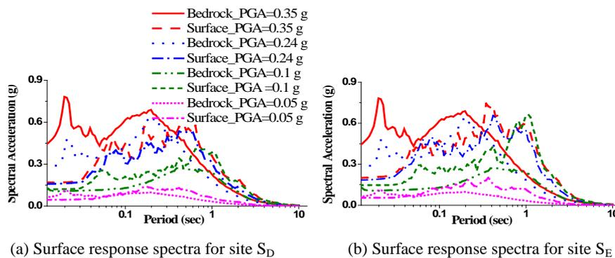
**Figure 14** The surface response spectra of several *PBA*s of input motion due to a megathrust earthquake with a return period of 2500 years.
