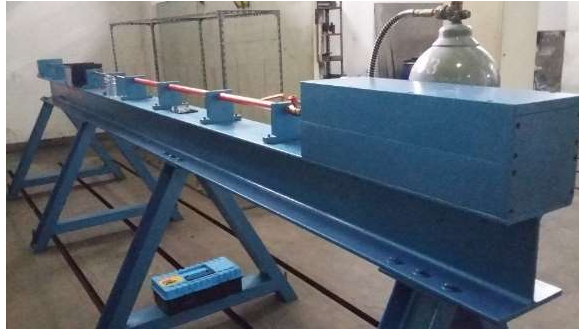
Figure 3 The SHPB in the Lightweight Structure Laboratory at ITB [31].
