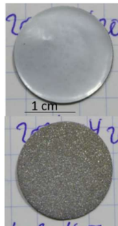
Figure 3 Metal-supported half-cell (SS, NiO-YSZ, and YSZ) sintered with different amounts of pore former but with an alumina lid with a space of 2 mm compared to the half-cells in Figure 1, which were sintered in open space without a lid.
