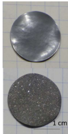
Figure 5 Metal-supported half-cell coated with carbon coating (stainless steel, NiO-YSZ, and YSZ) sintered with 3.7 g of pore former as described before in table 1 to 3 with tape-casting recipes, for a prolonged sintering time of 5 h at 1300 °C in open space.
