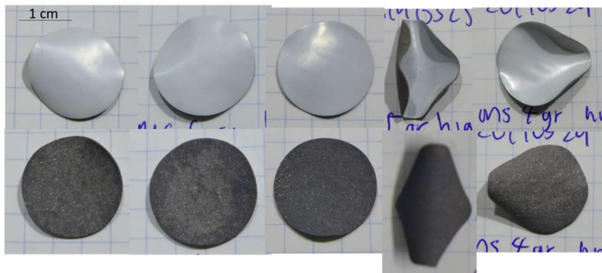
Figure 1 Metal-supported half-cell (stainless steel, NiO-YSZ, and YSZ) sintered with amount of pore former added varied at 7 g, 6 g, 5.5 g, 5 g, and 4 g, from right to left, as described before in tables 1 to 3 with tape-casting recipes for a sintering time of 5 minutes at 1300 °C.
