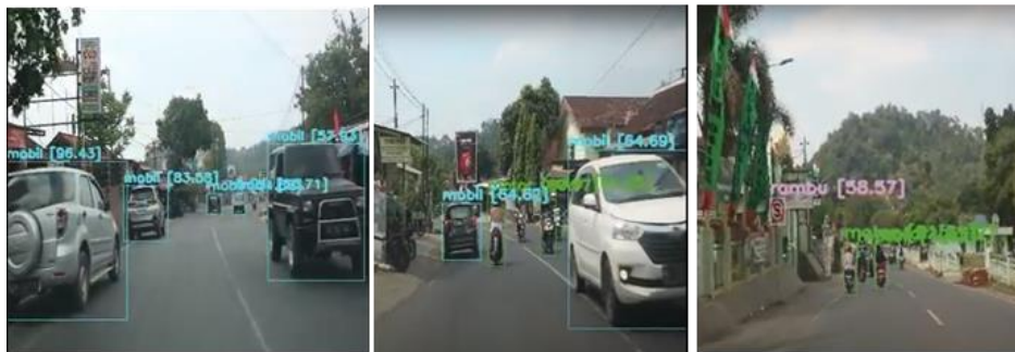
Figure 4 Accurate detection and recognition of all obstacles in a frame.
