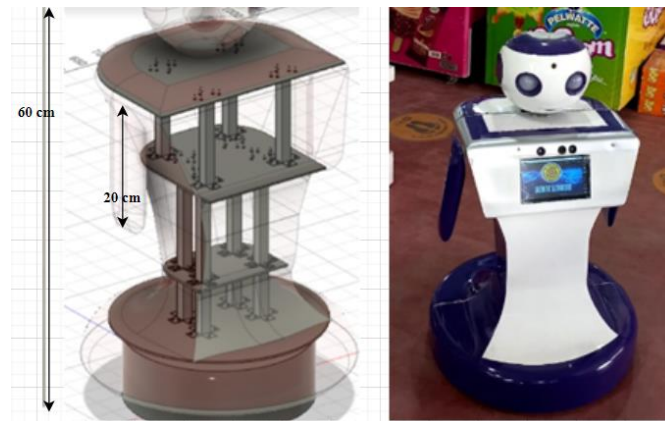
Figure 2 (a) Mechanical structure of the robot. (b) Finalized appearance.
