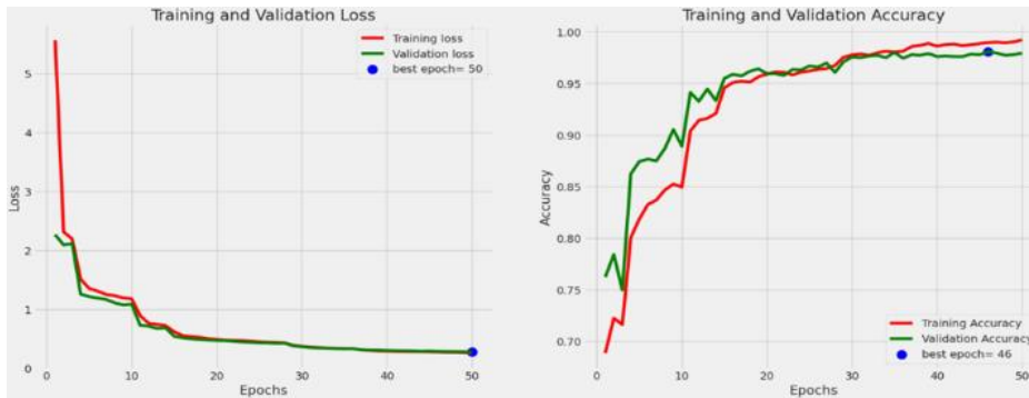
Figure 2 Training and validation loss and accuracy over 50 epochs for Inception V3.
