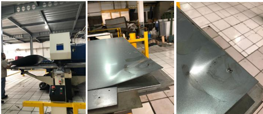
Figure 1 Stress material without tool optimization.
