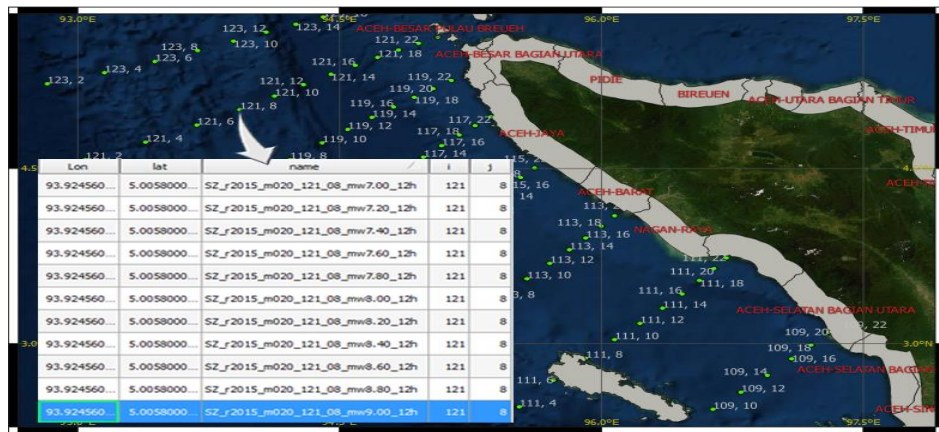
Figure 3 A small distribution of the Sunda Zone (SZ) tsunami simulation scenario, which also represents the position index of the scenario in its fault zone with the values of i and j .
