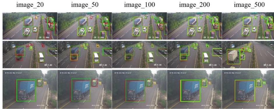
Figure 6 Visual comparison for object detection. Red: Ground truth, green: SSD, yellow: YOLO.
