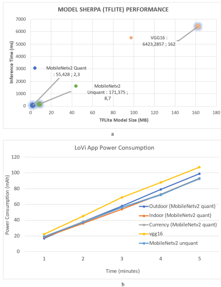
Figure 9 Test results of (a) the inference time and size of the Sherpa model, and (b) the smartphone power consumption by the LoVi app.
