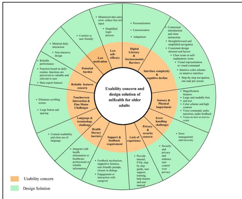
Figure 4 Visual representation mapping usability concerns to design solutions in mHealth applications for older adults.
