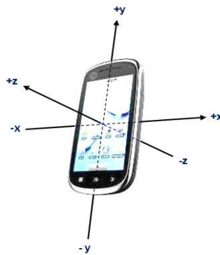
Figure 1 Coordinate system of the motion sensors.
