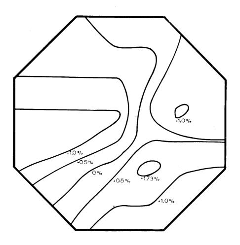
Figure 3. Velocity Contour at the Test Section, 20 cm downstream of the center Section. Average velocity 30.13 m/sec with standard deviation of 0.70%.
