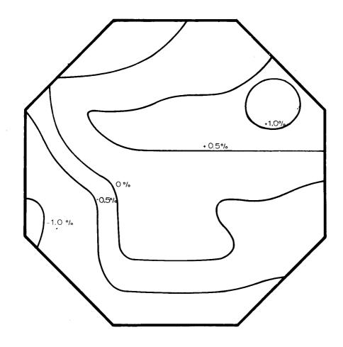
Figure 2. Velocity Contour at the Test Section measured at the center of the Test Section. Average velocity = 30.15 m/sec with standard deviation of = 0.45%.
