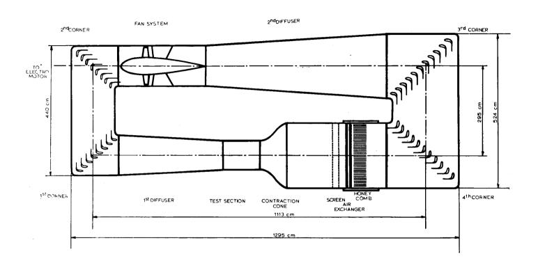
Figure 1. Schematic Diagram, Wind-Tunnel.
