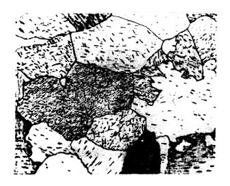
Figure 7. Microstructure of 20.0 wt % Sn alloy Furnace cooled from 400°C; mag. 400 X
