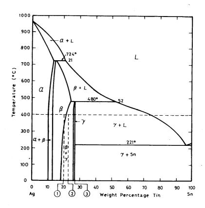
Figure 1. Phase diagram of Ag-Sn system
