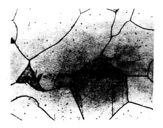
Figure 2. Microstructure of  $\gamma$  phase or Ag<sub>3</sub>Sn Furnace cooled from 400°C; mag. 400 X
