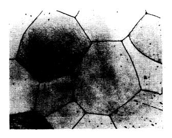
Figure 3. Microstructure of  $\gamma$  phase or Ag  $_3Sn$   $_2$  Quenched in water from 400°C; mag. 400 X
