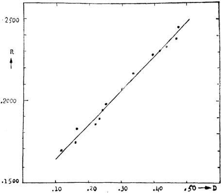
Fig. 2. Relationship between Astrophotometer Reading and Emulsion Density.
