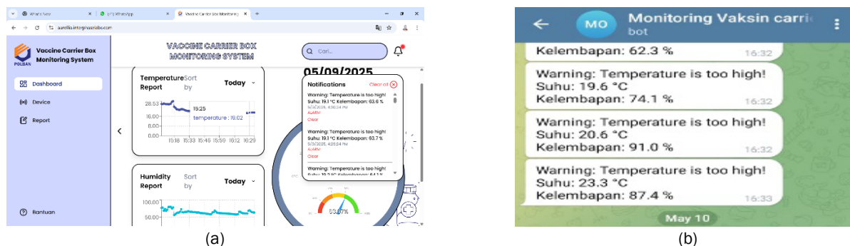
Figure 9. Example of automatic alarm notifications sent via: (a) Web Dashboard, (b) Telegram Interface
