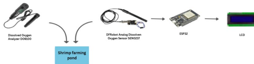
Figure 4. DFRobot analog dissolved oxygen sensor SEN0237 validation scheme.
