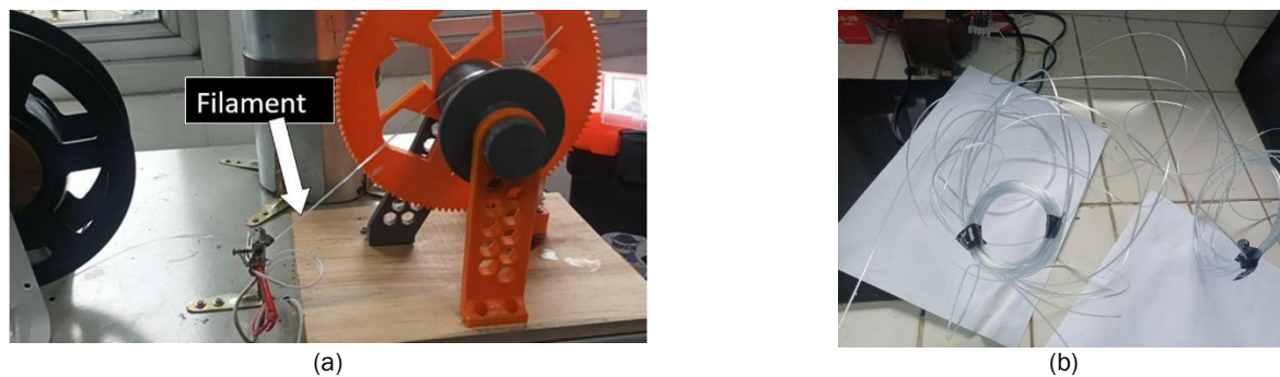
Figure 8. (a) Filament processing in the pultrusion machine; (b) PET bottle filament.
