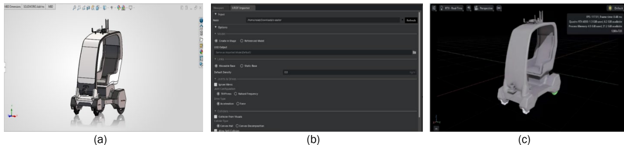
Figure 2. Stages of converting the O-SEATER virtual model: (a) CAD model in SolidWorks, (b) conversion process using URDF Importer, and (c) O-SEATER model in USD format on NVIDIA Isaac Sim.
