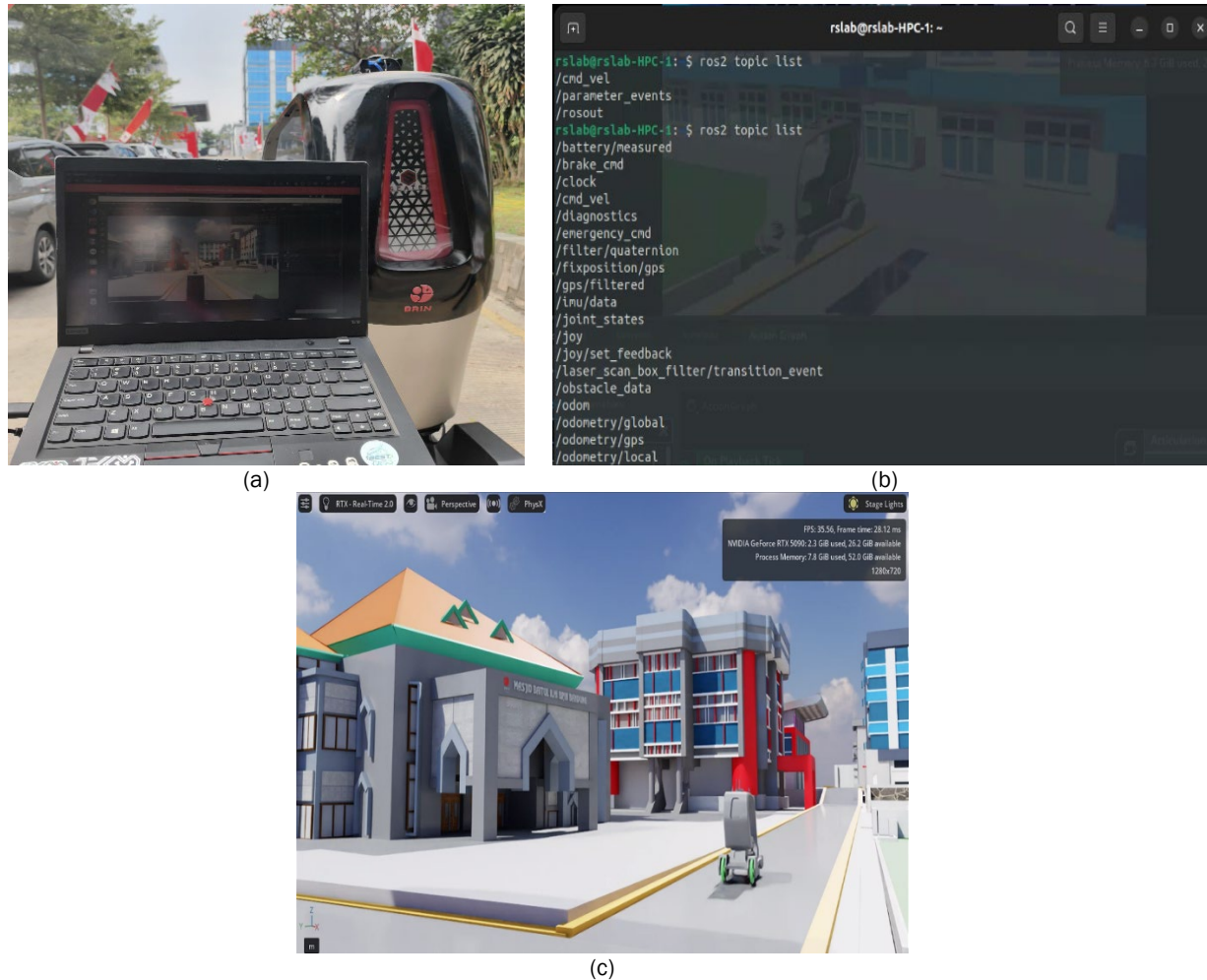
Figure 13. Hardware-in-the-Loop Implementation (a) the operator controls the O-SEATER using a joystick, (b) results of ROS 2 communication integration between the actual and virtual O-SEATER, and (c) the virtual O-SEATER in the NVIDIA Isaac Sim simulation environment responding to control commands.
