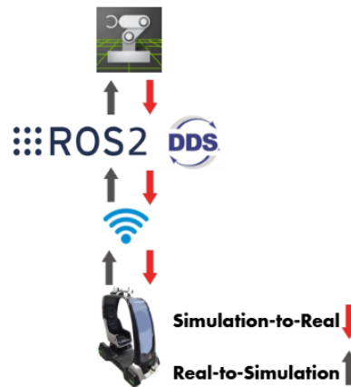
Figure 6. Communication architecture between the actual O-SEATER and the simulation platform using ROS 2 based on DDS over a Wi-Fi network
