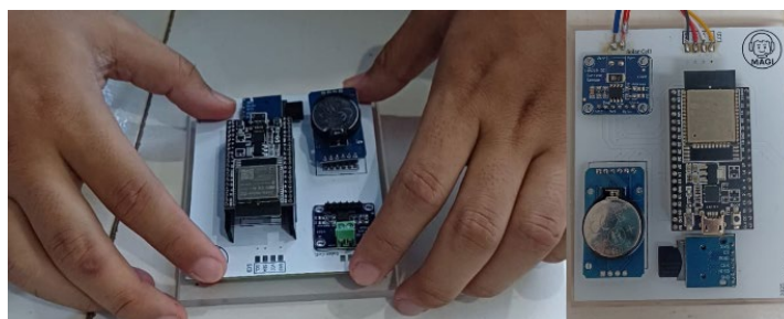
Figure 8. Hardware components installation on custom PCB
