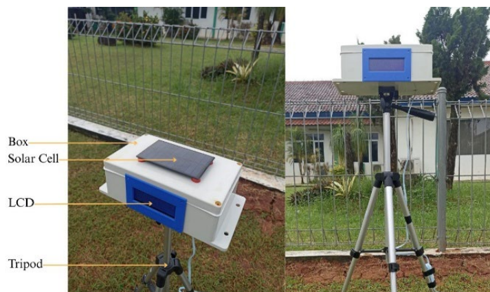
Figure 9. Box and tripod installation
