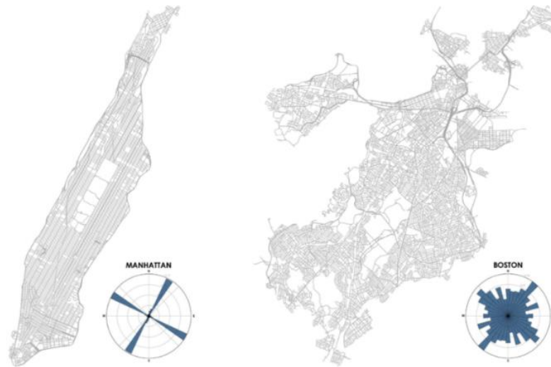
Figure 4. OSMnx provides not only a visual representation of formal/grid patterns or natural/organic patterns, but also topological configuration analytics. Source: Boeing, 2019
