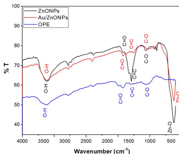
**Figure 1.** FTIR spectra of ZnONPs, Au/ZnONPs, and orange peel extract (OPE)
