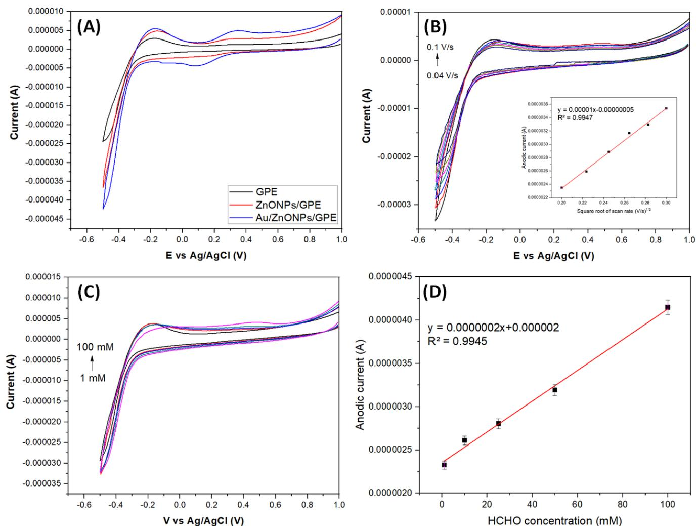
**Figure 3.** (A) The Cyclic voltammograms of 25 mM formaldehyde in 0.1 M phosphate buffer pH 9 on Au/ZnONPs/GPE compared to ZnONPs/GPE and bare GPE electrode; (B) the effect of scan rate against the CVs profile of the formaldehyde on Au/ZnONPs/GPE; (C) the effect of formaldehyde concentrations and (D) its linear correlation against the anodic current at 0.36 V extracted from (C)
