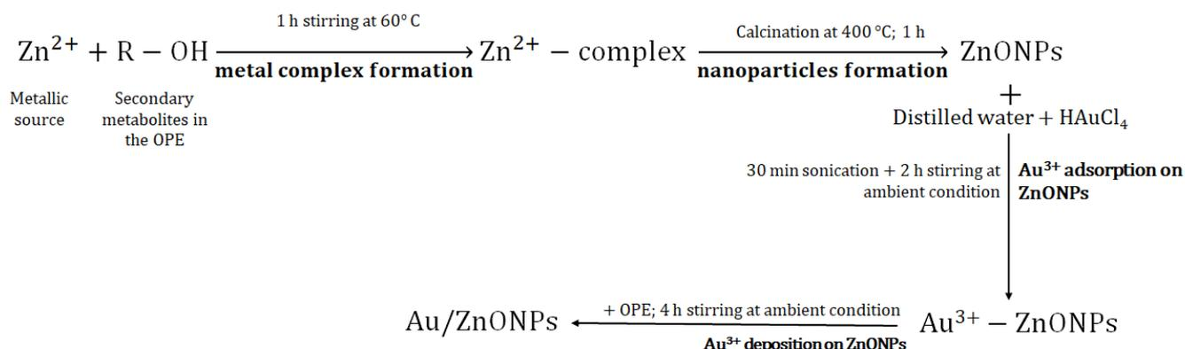
**Scheme 1.** The proposed mechanism of Au/ZnONPs formation
