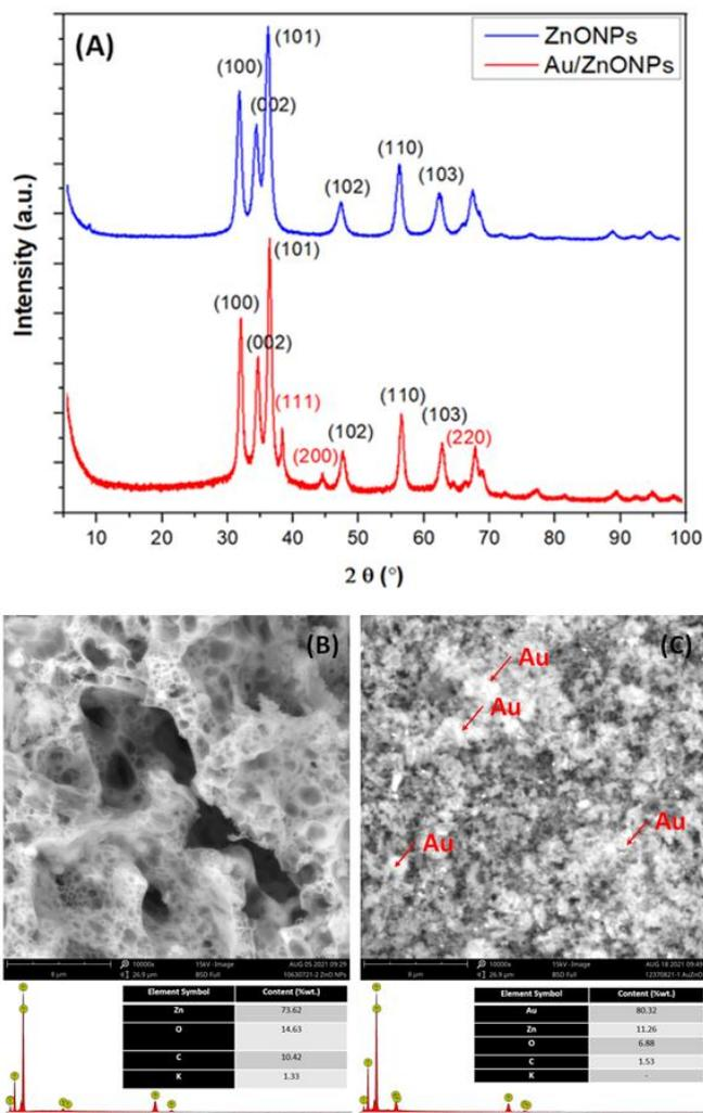
**Figure 2.** (A) XRD pattern; (B) and (C) SEM-EDX profile of ZnONPs and Au/ZnONPs, respectively
