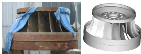
Gambar 7. Model digital dan model fisik runner
