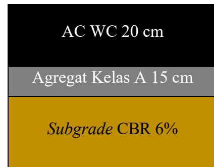
Figure 3. Existing pavement structure
