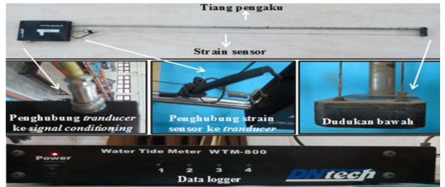
Gambar 4. Wave Probe Seri WTM-800 v2
