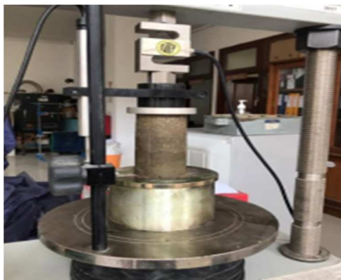
Gambar 6. Pengujian kuat tekan bebas (unconfined compression strength test)
