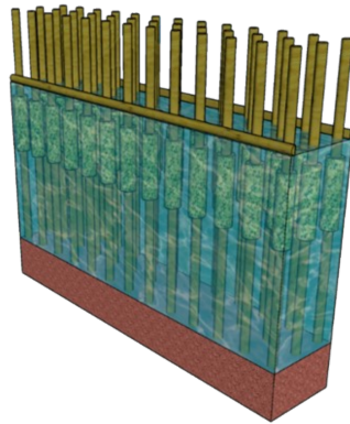
Figure 4. Three-dimensional design of a 5 x 1 m coastal protection structure
