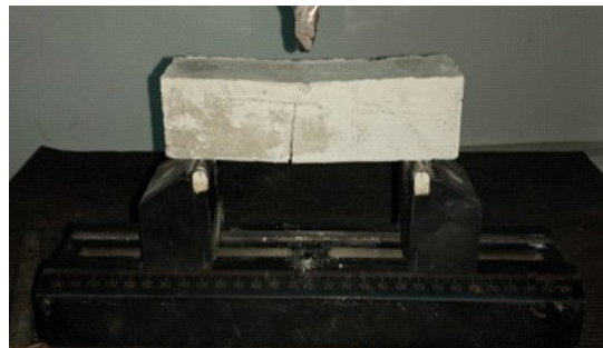
Gambar 1. (a) Mesin uji kuat lentur UTM, (b) sample uji kuat lentur
