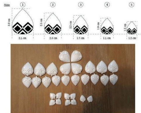
Figure 10 Size and prototype work in centrifugal casting, Activity 2.
