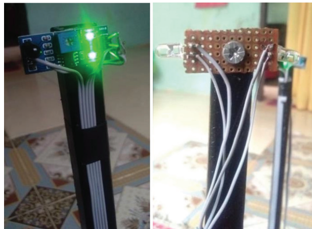
Figure 4 Photodiode and infrared sensor installation
